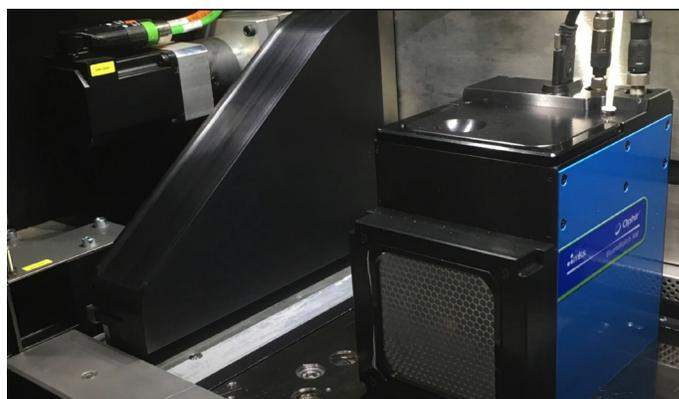
Ophir BeamWatch AM high-power beam profiler integrated into a PBF system
