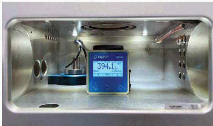
Ophir Ariel laser power sensor inside a small build chamber
